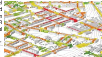
Work-in-progress generating the street sections: top and oblique view with sections displayed corresponding to their width and height, classified according to gaps between buildings (green = many to red = few)
