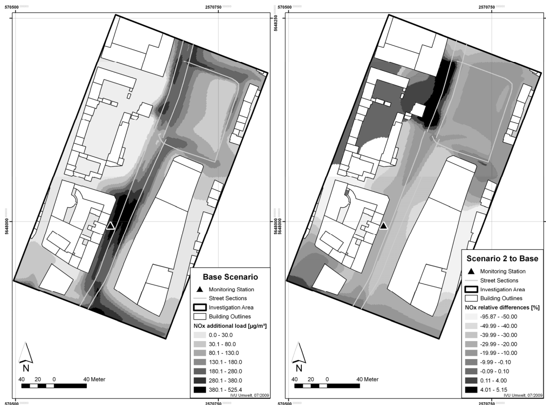
Figure 4: Left: NO x additional pollutant load due to traffic emissions under critical wind direction 270° for Clevischer Ring at level 1.3 m – 2.0 m, Base Scenario. Right: Relative differences of NO x additional pollutant load, Scenario 2 to Base Scenario.
